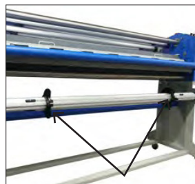
Media alignment disks keep supply rolls from telescoping.
