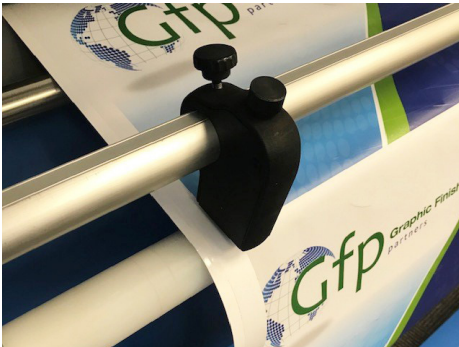
Inline Rotary Slitters: Trims output during lamination to save time
