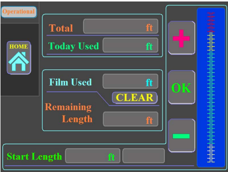
Film Usage Counter: Tracks film usage per job, per day, and lifetime.
